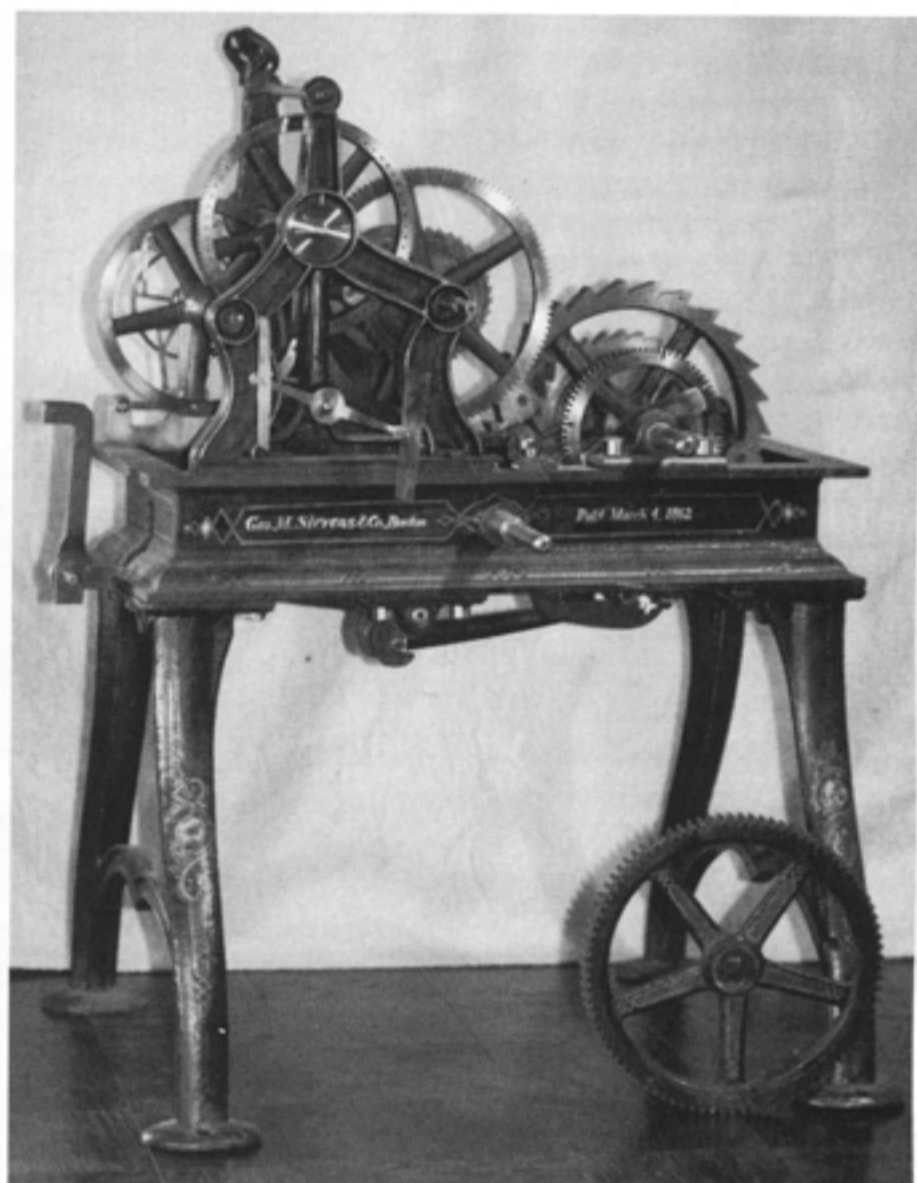
GMS Figure 1. GMS Model 1 front overview, time left, strike right. Note the time free-form A-frame, its inset setting dial, and the escapement remontoire fly. The crane-striker ratchet and associated wheels are on a single arbor wound with winding jack aid, its wheel seen at bottom right.
