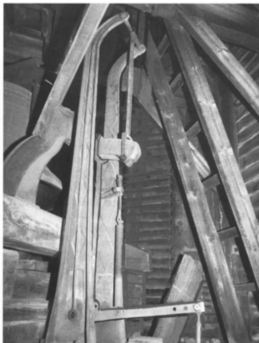
GMS Figure 3. Model 2 overview. The crane-striker with a winding jack has been retained but its steel weight line winding barrel requires a Stevens hallmark, the frame offset. The time train is a complete redesign, including its cast-iron A-frame with Vuillamy bushings, Harrison maintaining, and a four-wheel train with Graham deadbeat escapement. Precision pendulum rating and beat adjustments are provided.
